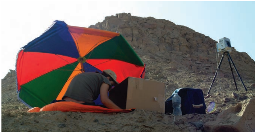
Fig. 21.3 Fieldwork with the laser scanner: The laptop is protected against dust and sunlight by a cardboard box
